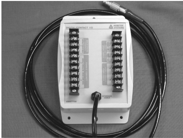
Figure 1.8: External I/O Module and Cable Assembly
